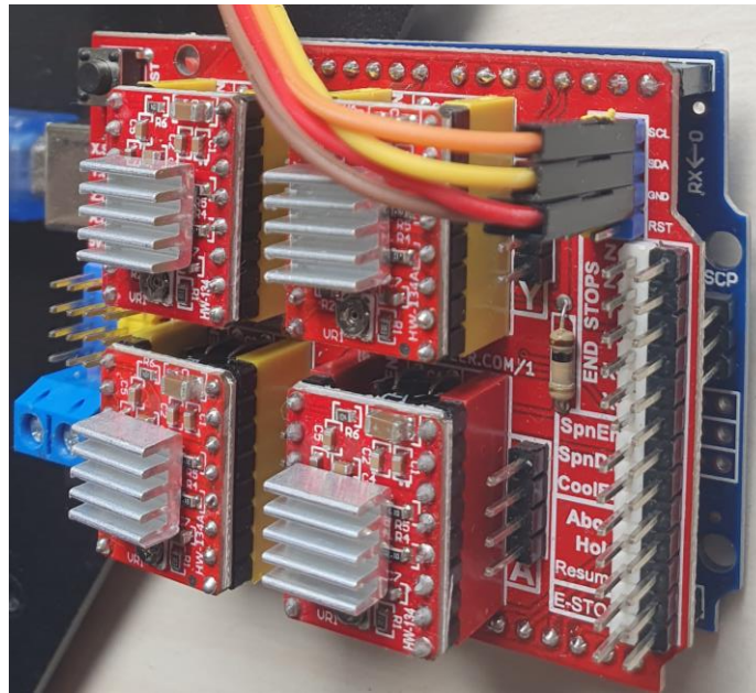
Figure 44. CNC Shield with Four A4988 Stepper Drivers
